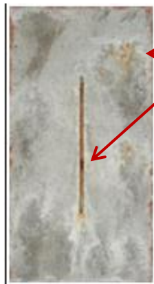
Layer Thickness: 4.1 mils Adhesion: 5,187 psi
