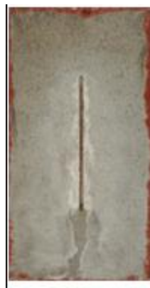
Layer Thickness: 12.7 mils Adhesion: 3,375 psi
