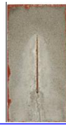
Layer Thickness: 24.5 mils Adhesion: 2,519 psi
